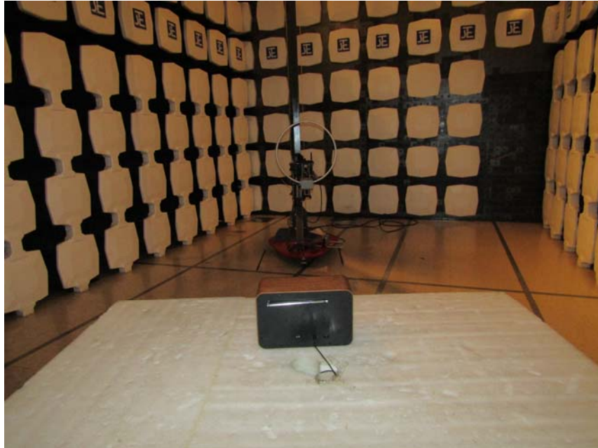
Measurement of Radiated Emission Test Set Up
