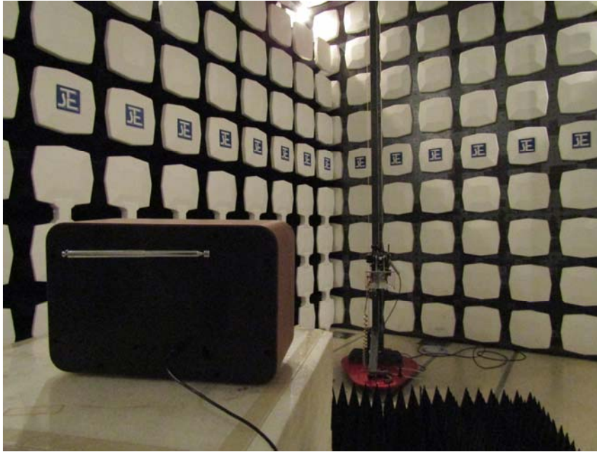
Measurement of Radiated Emission Test Set Up
