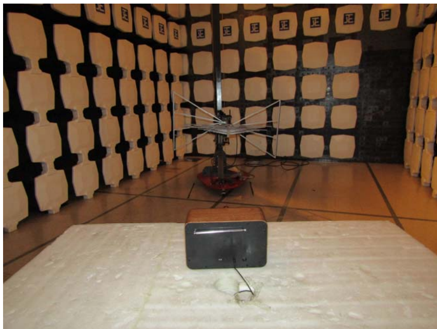
Measurement of Radiated Emission Test Set Up
