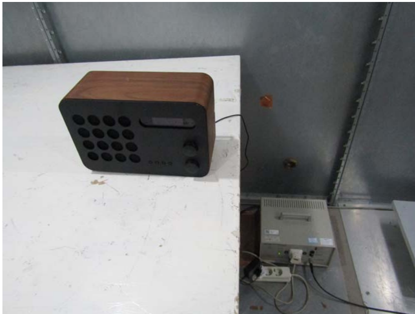
Measurement of Conducted Emission Test Set Up
