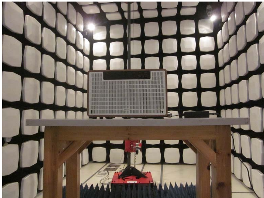
Measurement of Conducted Emission Test Set Up
