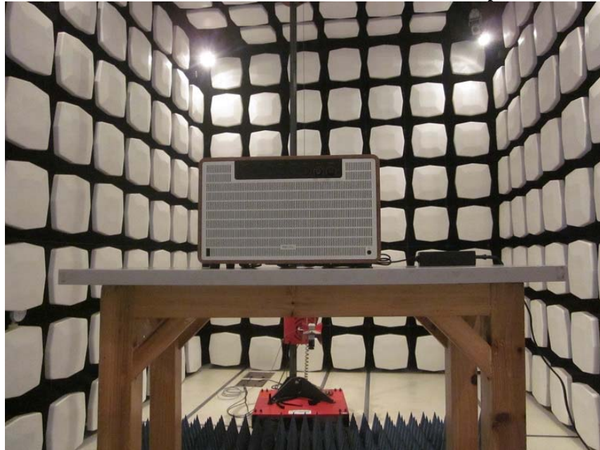
Measurement of Radiated Emission Test Set Up
