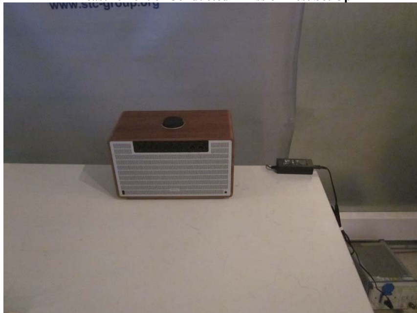
Measurement of Conducted Emission Test Set Up
