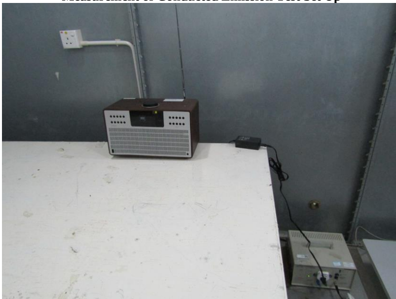
Measurement of Conducted Emission Test Set Up
