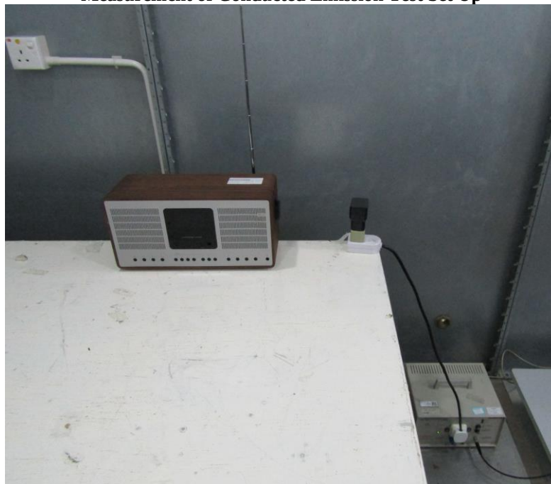
Measurement of Conducted Emission Test Set Up
