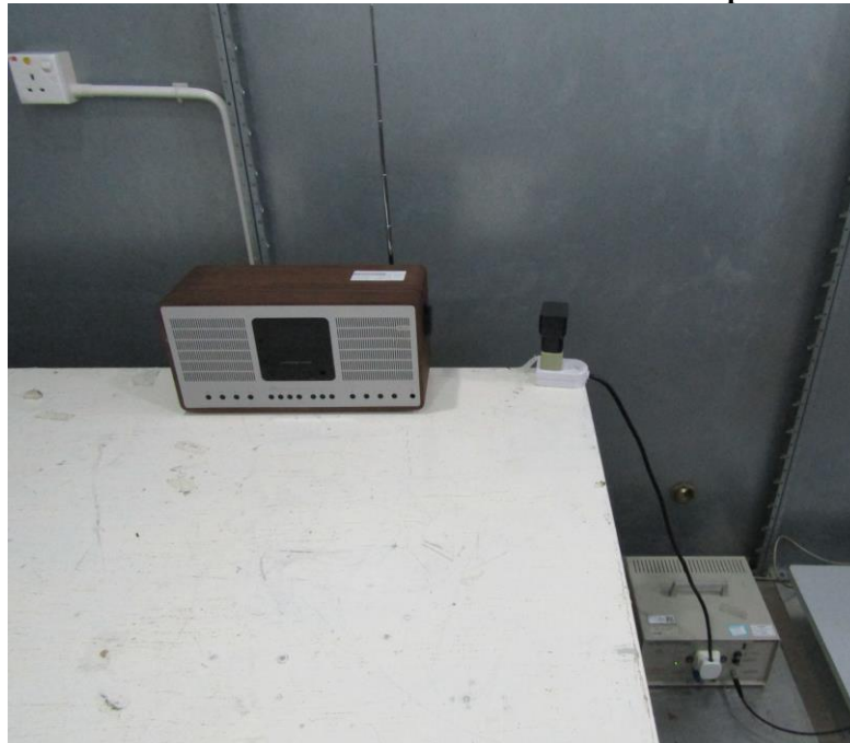
Measurement of Conducted Emission Test Set Up
