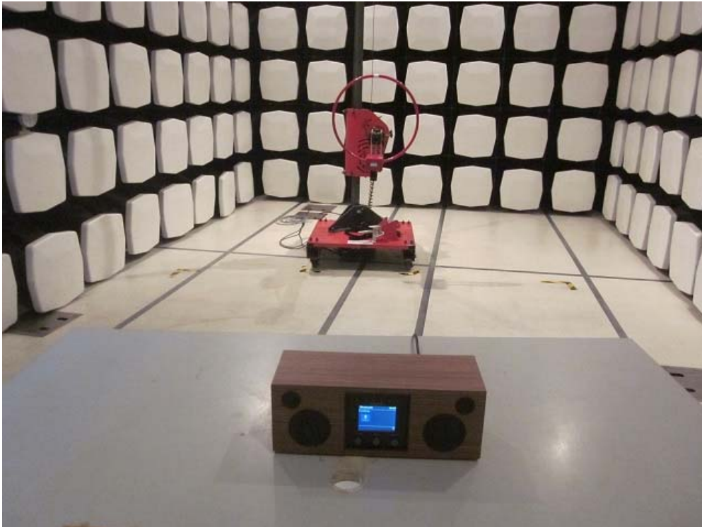
Measurement of Radiated Emission Test Set Up
