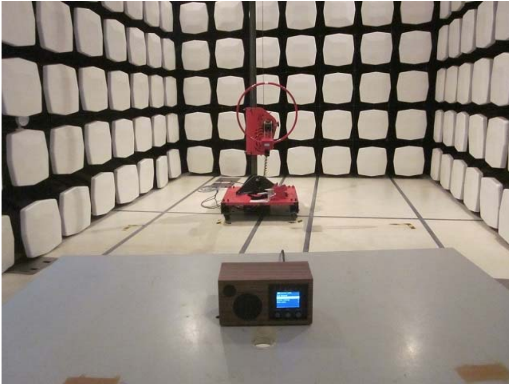
Measurement of Radiated Emission Test Set Up
