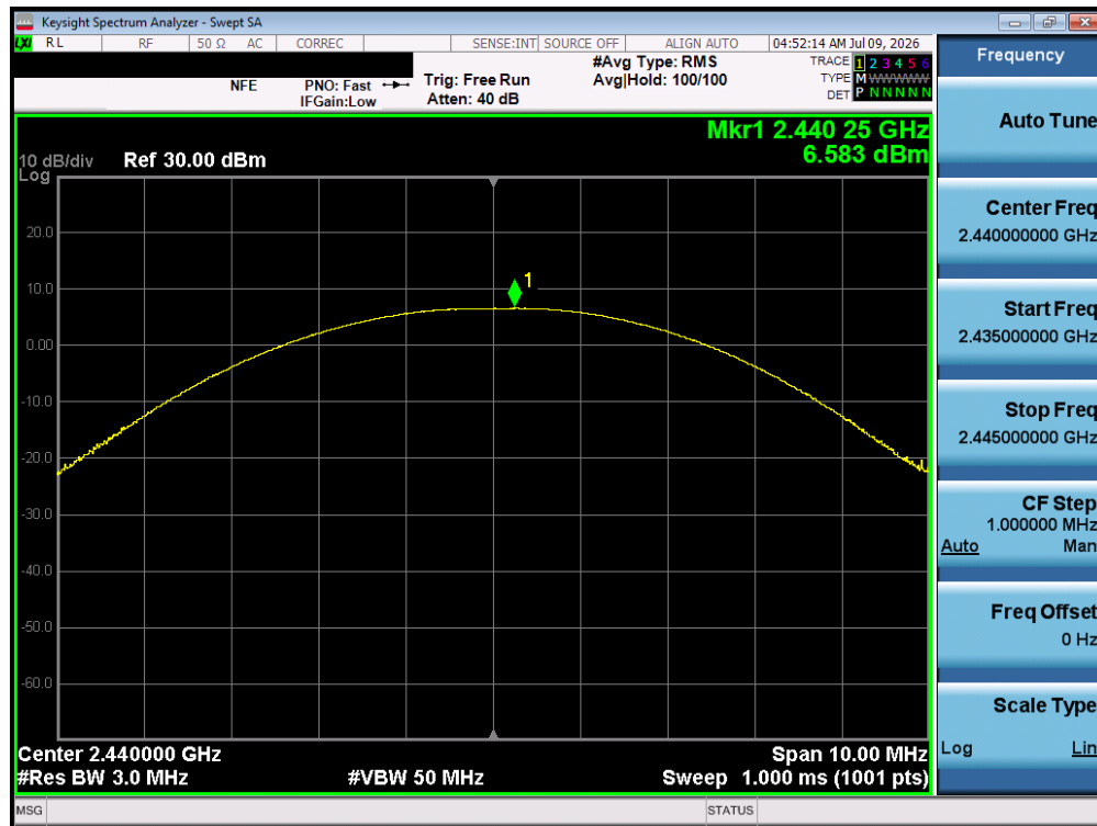
Plot 7-14. Peak Power Plot (Bluetooth (LE), 500kbps – Ch. 17) – MIMO Ant1
