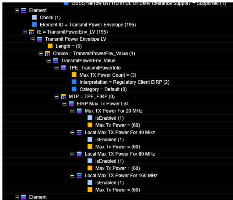
Figure 7-2. Callbox Power Authorization – 36.00dBm
