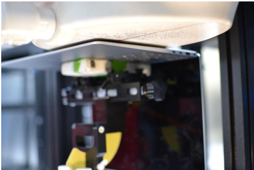
SAR Test Setup Photo 1 – Motion, Bottom Side at 0 mm – Antenna 1 & 2
