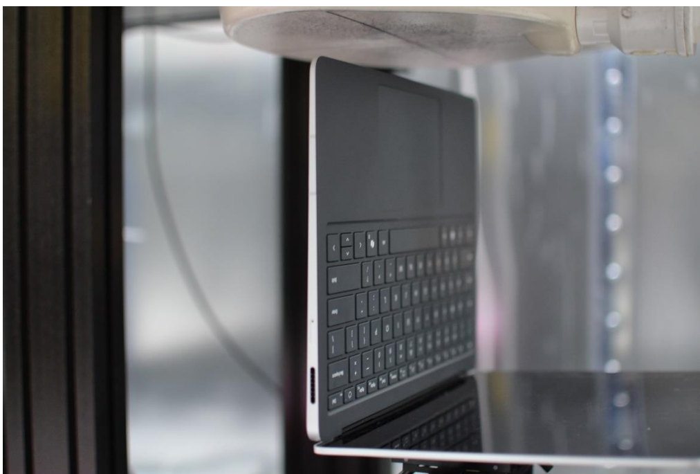
SAR Test Setup Photo 12 – No Motion, Front Edge at 25 mm – Antenna 3 & 4
