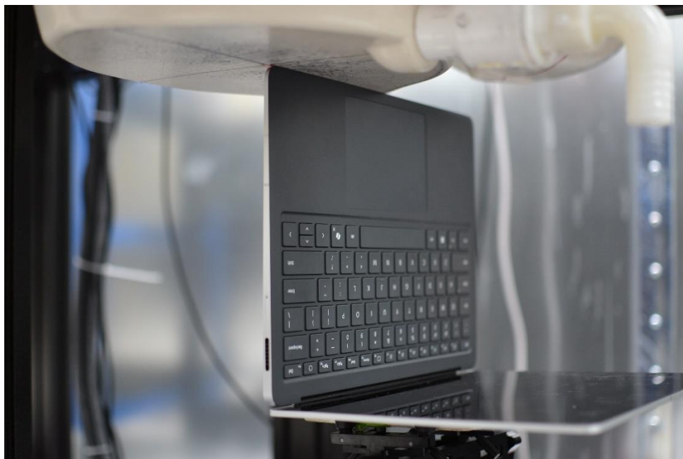
SAR Test Setup Photo 13 – Motion, Front Edge at 0 mm – Antenna 5 & 6
