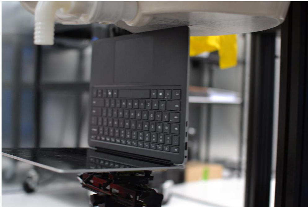
SAR Test Setup Photo 9 – Motion, Front Edge at 0 mm – Antenna 1 & 2
