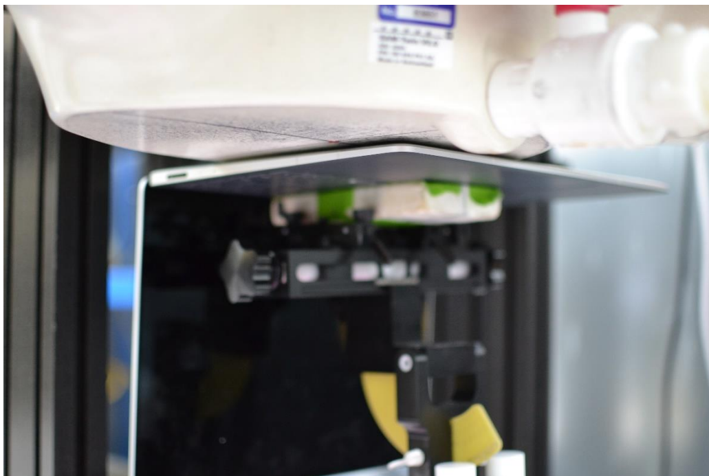
SAR Test Setup Photo 5 – Motion, Bottom Side at 0 mm – Antenna 5 & 6
