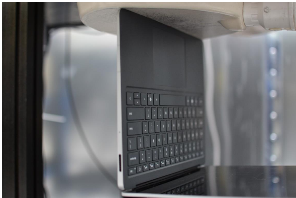
SAR Test Setup Photo 11 – Motion, Front Edge at 0 mm – Antenna 3 & 4
