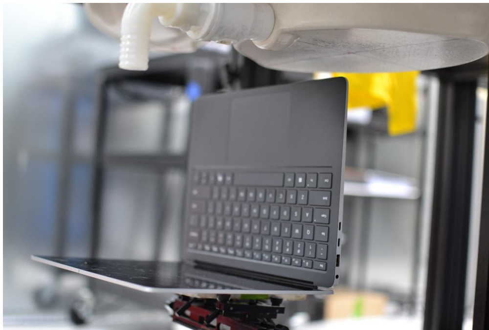
SAR Test Setup Photo 10 – No Motion, Front Edge at 25 mm – Antenna 1 & 2
