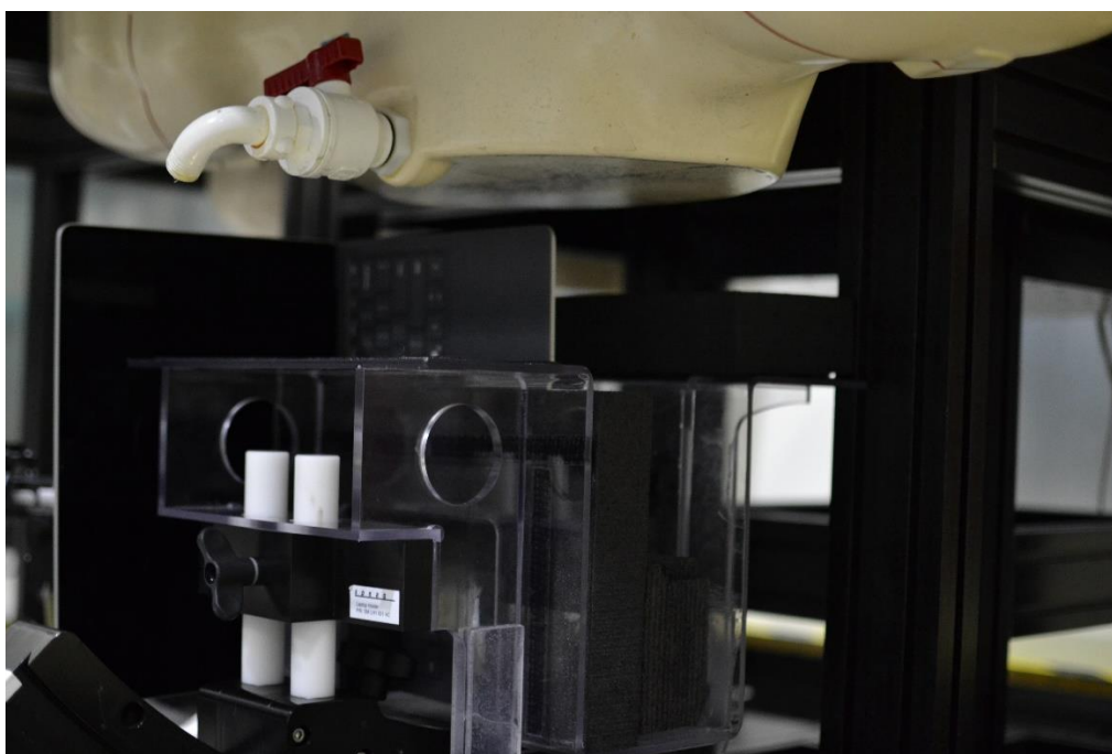
SAR Test Setup Photo 18 – No Motion, Right Edge at 25 mm
