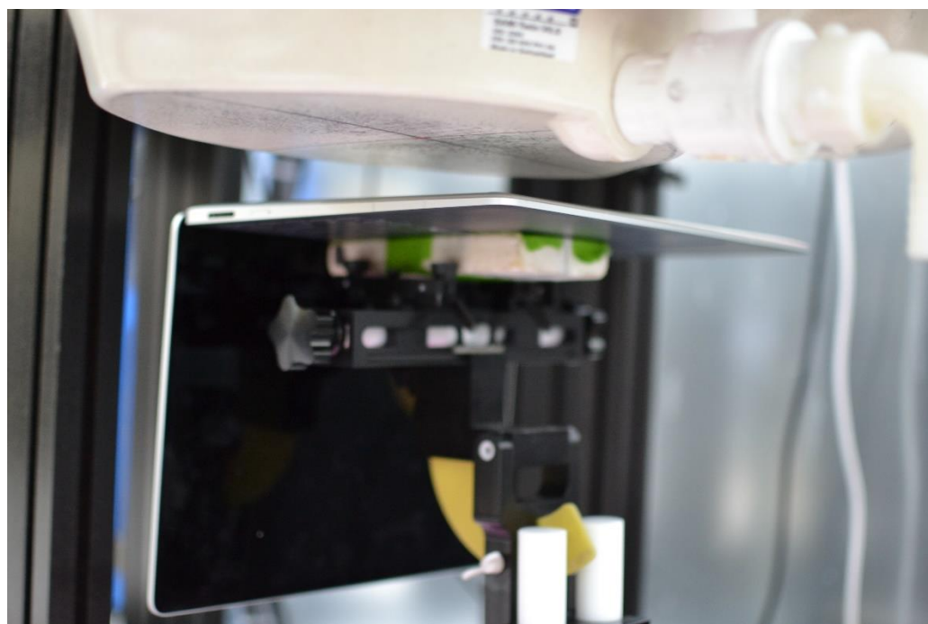
SAR Test Setup Photo 6 – No Motion, Bottom Side at 25 mm – Antenna 5 & 6
