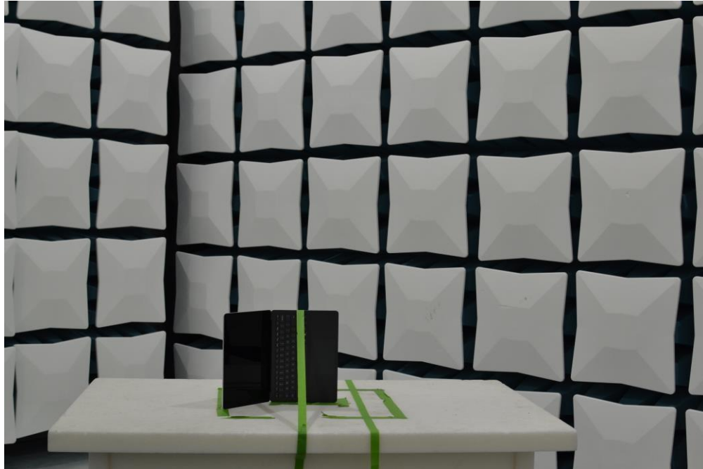
Figure 13. Test Setup – Y Position – 30MHz-1GHz – Open
