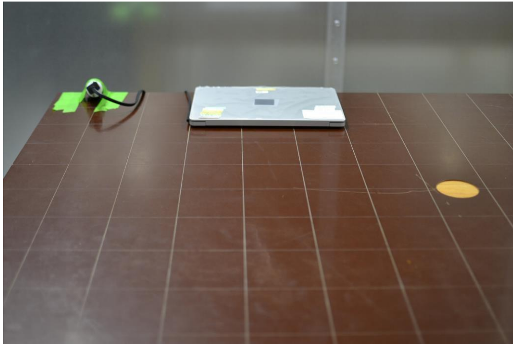
Figure 1. Test Setup – ACLC– <30MHz
