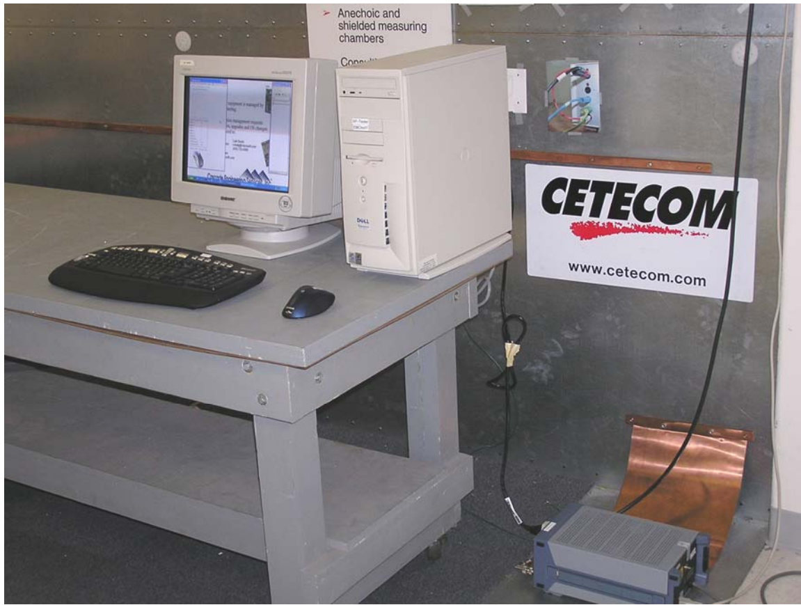
Test setup – AC Line conducted emissions
