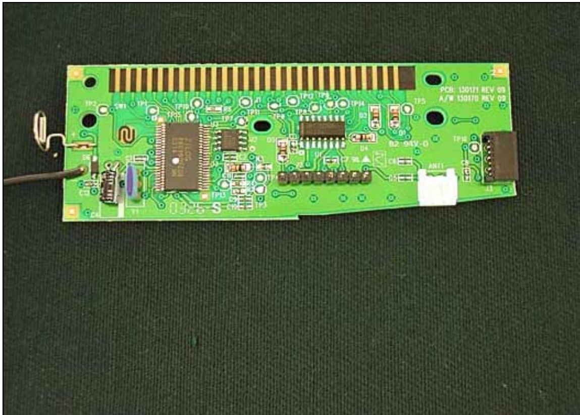
Keyboard - Main PCB Bottom Side
