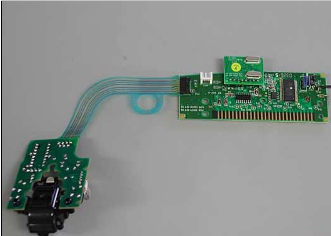
Keyboard - Bottom of 3 PCBs
