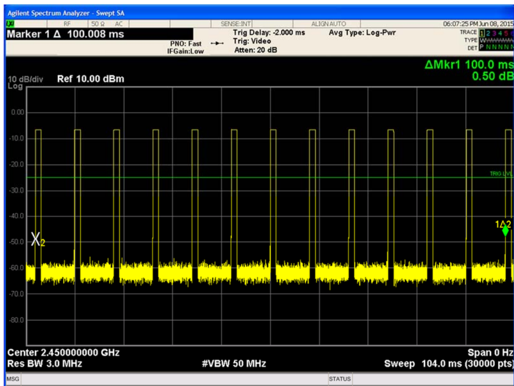
Figure 9-2 Pulse Train over 100ms
