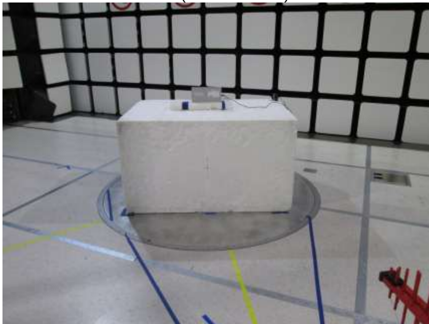
RADIATED BACK PHOTO (BELOW 1 GHz)
