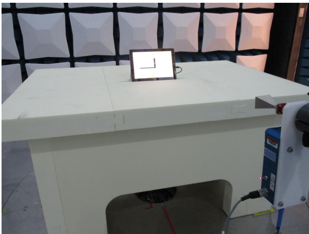
Fig.4 Radiated Spurious Emissions (18-26.5GHz)
