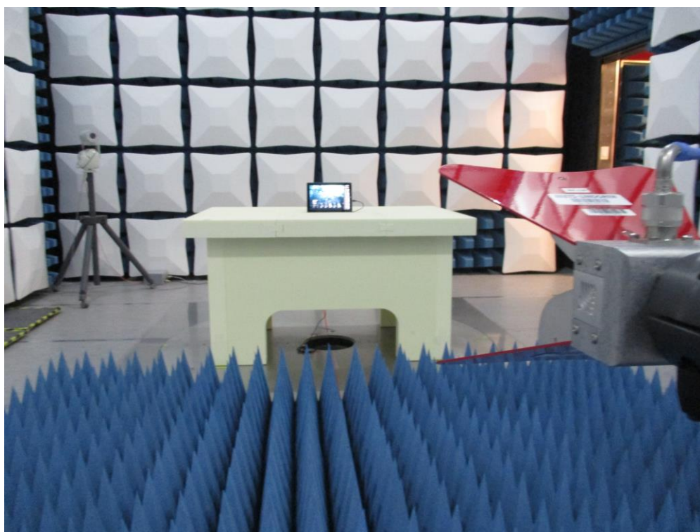
Fig.3 Radiated Spurious Emissions Test Setup (1-18 GHz)
