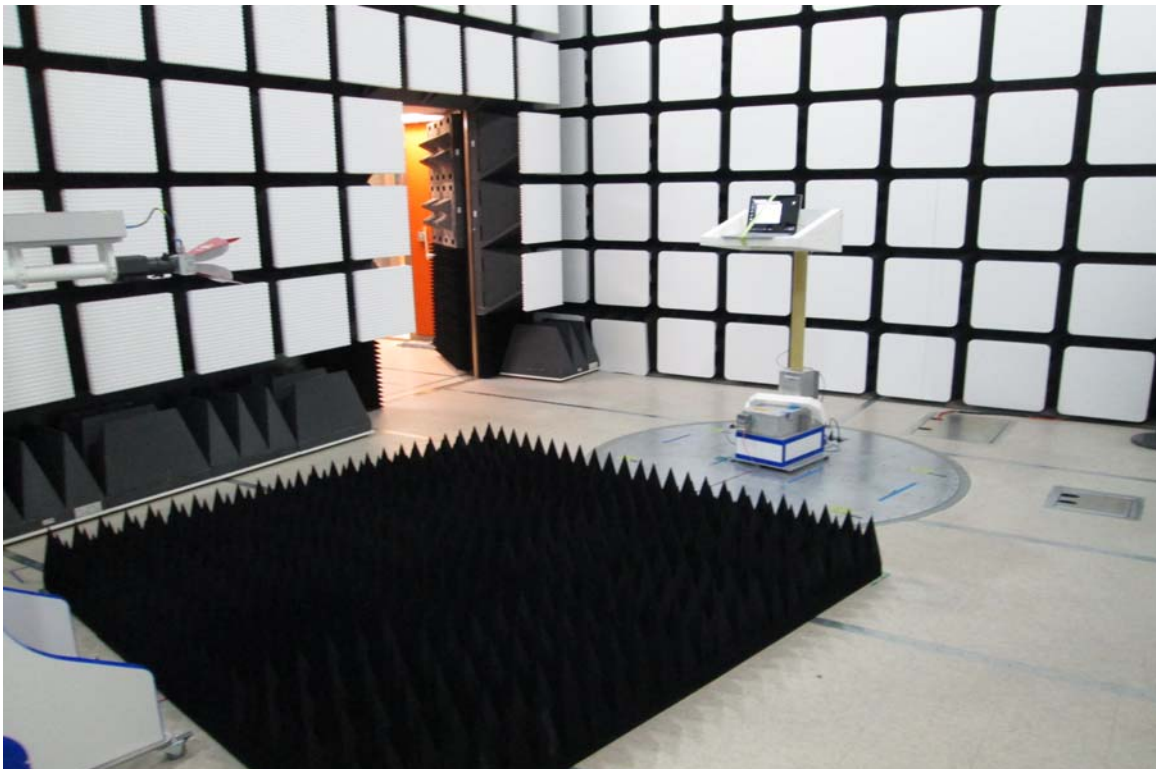
Fig.2 Radiated Spurious Emissions Test Setup (1-18 GHz)
