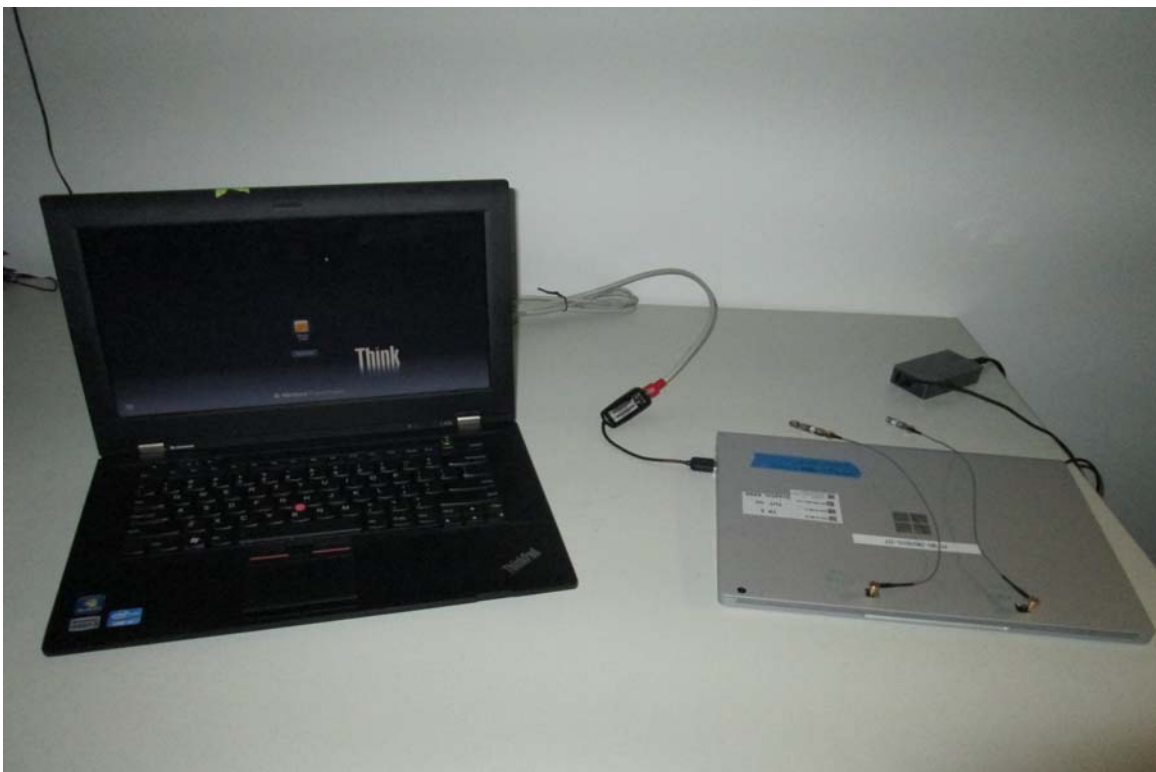
Fig.4 Antenna port Conducted Measurements Test Setup
