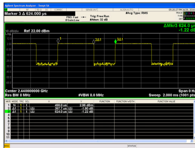
Figure 9-2. Duty Cycle 2440MHz (Ch.19)
