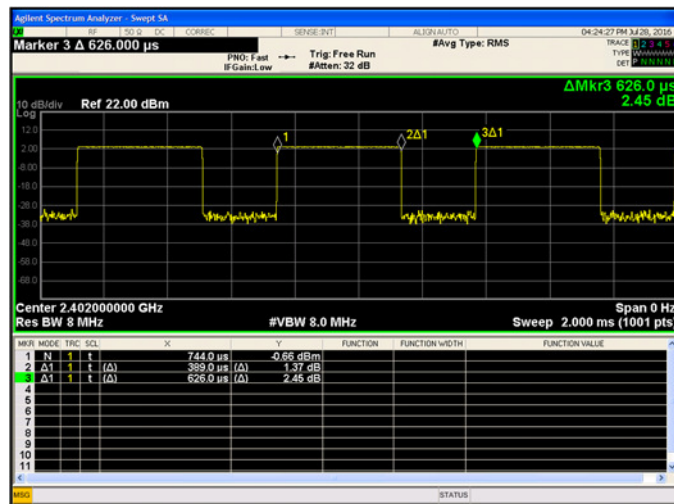
Figure 9-1. Duty Cycle 2402MHz (Ch.0)
