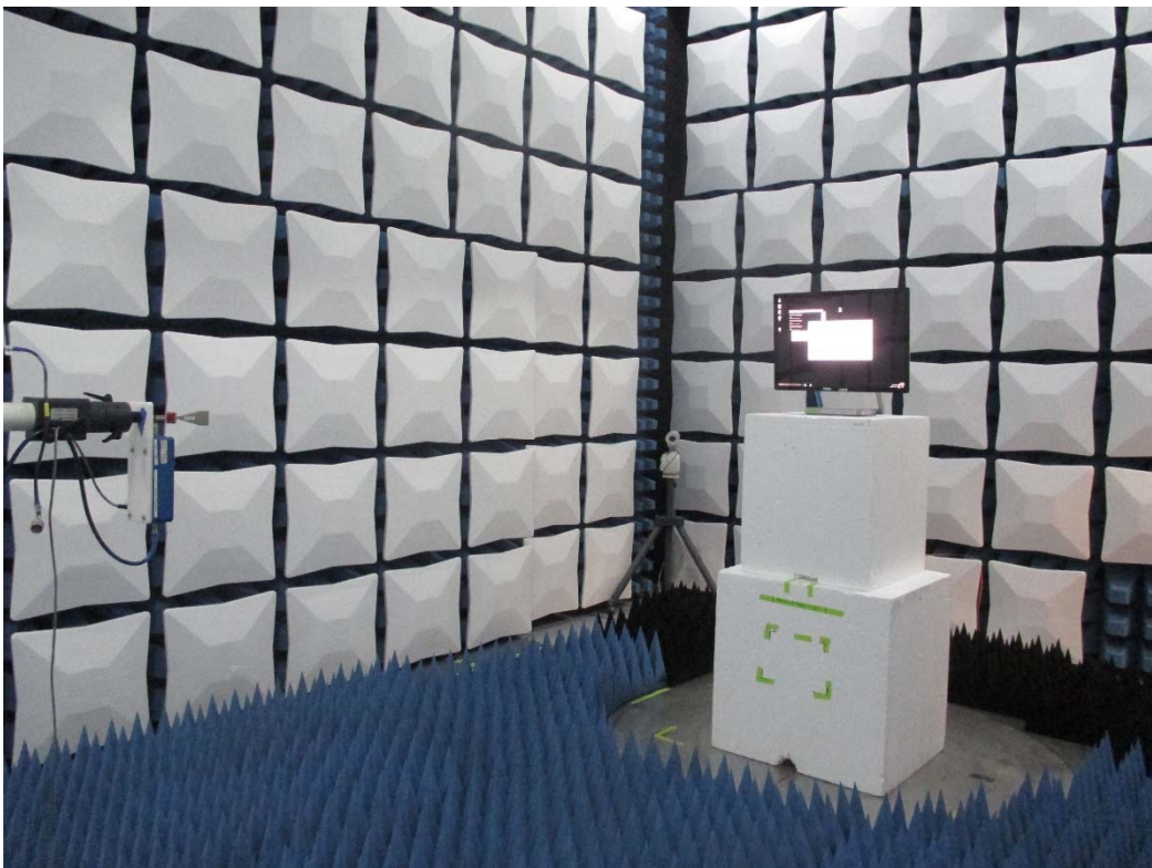
Fig.4 Radiated Spurious Emissions (18-26.5GHz) Test Site2
