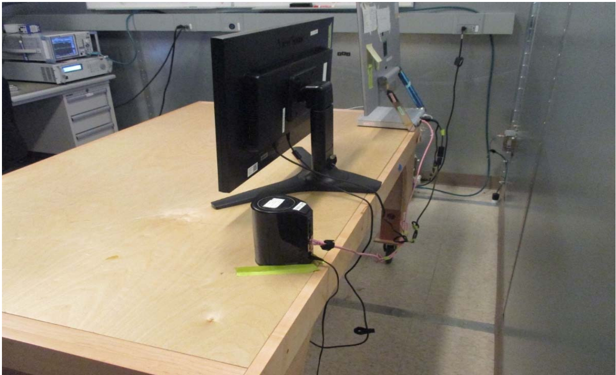
Fig.9 AC Line Conducted Emissions Measurements Test Setup- Back View
