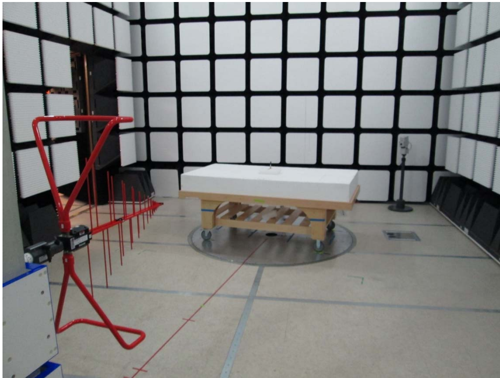
Fig.3 Radiated Spurious Emissions Test Setup (30MHz – 1GHz)
