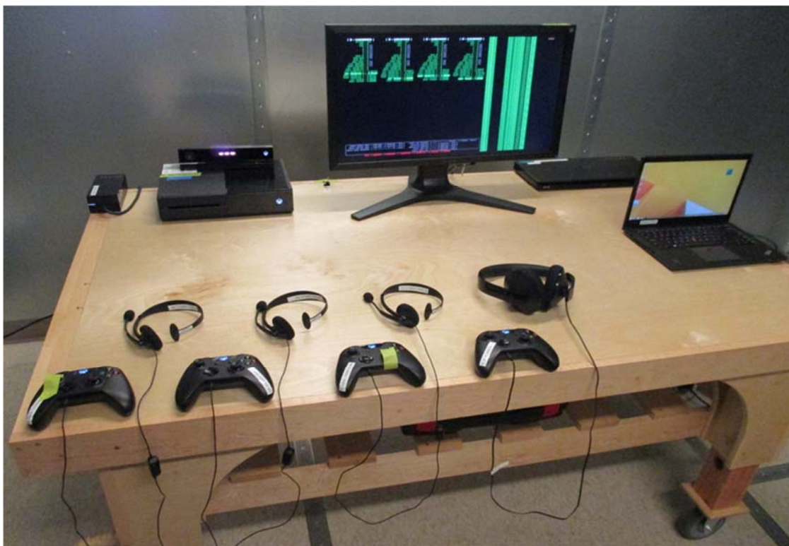
Fig.9 AC Line Conducted Emissions Measurements Test Setup
