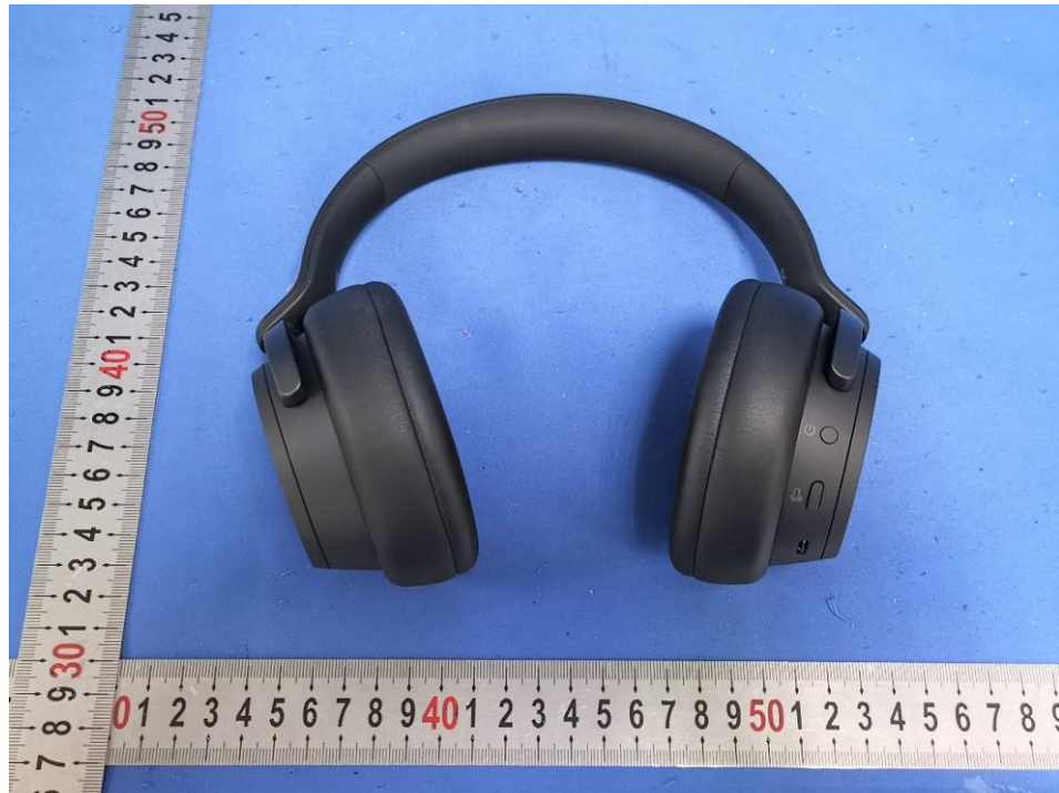
Right Earcup has power, mute buttons and charging port
