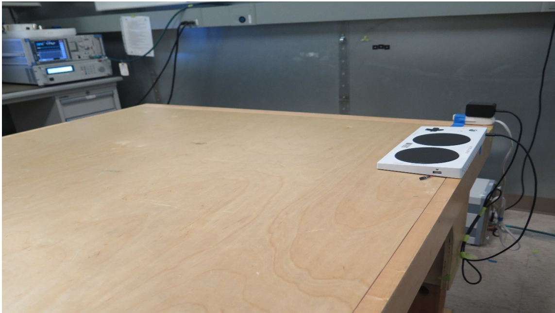
Figure 7 AC Line Conducted Emissions Test Setup -Side View
