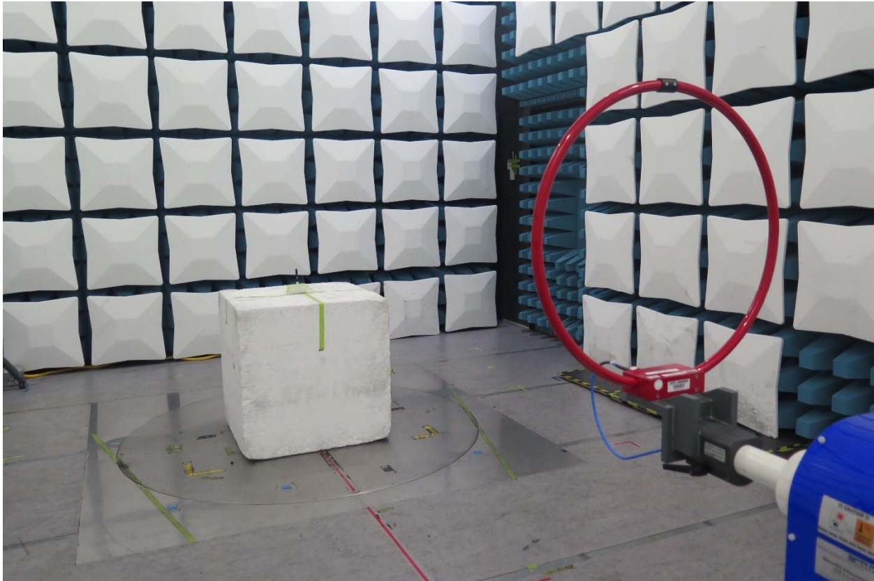
Figure 1 Radiated Spurious Emissions Test Setup (9KHz-30MHz)
