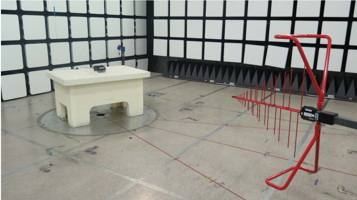
Figure 1 Radiated Spurious Emissions Test Setup (30M-1GHz)
