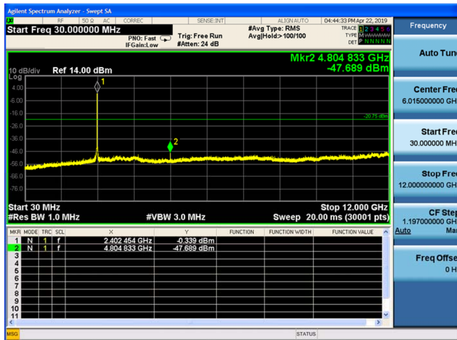
Figure 9-15 Conducted Spurious Emissions 30-12000 MHz (Ch. 0)
