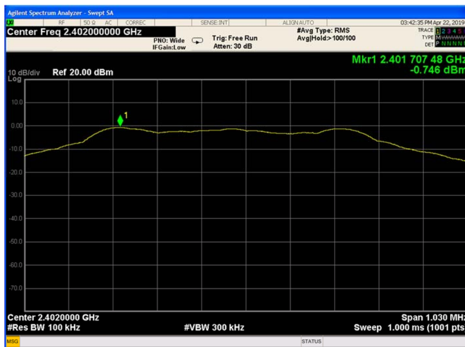
Figure 9-14 Reference Level Measurement (Ch.0)
