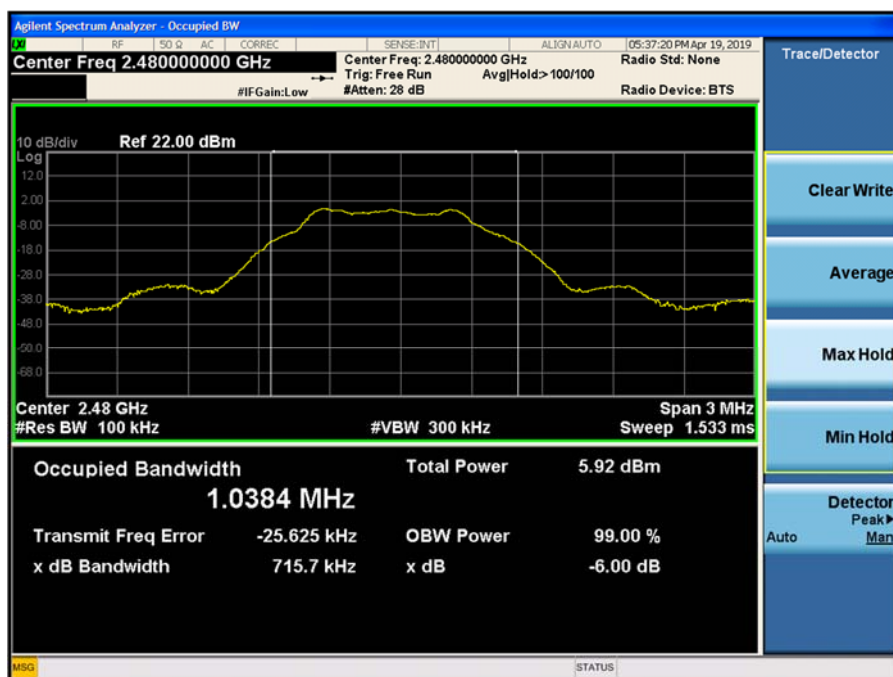
Figure 9-4 6dB Bandwidth (Ch. 39)
