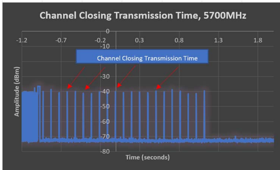
Figure 27. Channel Closing Transmission Time (5700MHz), 20MHz Bandwidth
