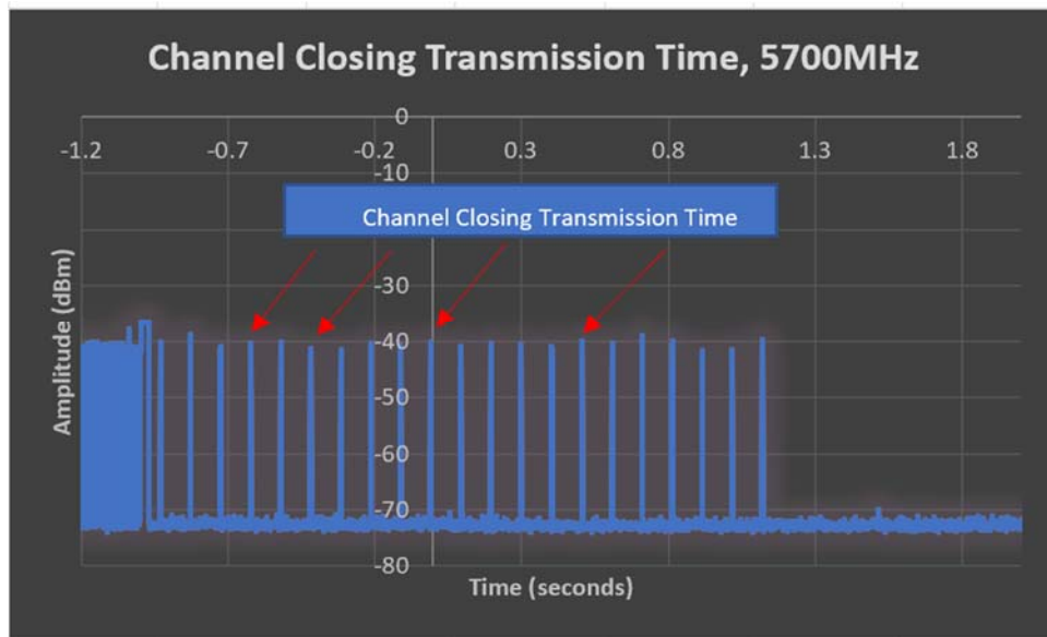
Figure 27. Channel Closing Transmission Time (5700MHz), 20MHz Bandwidth
