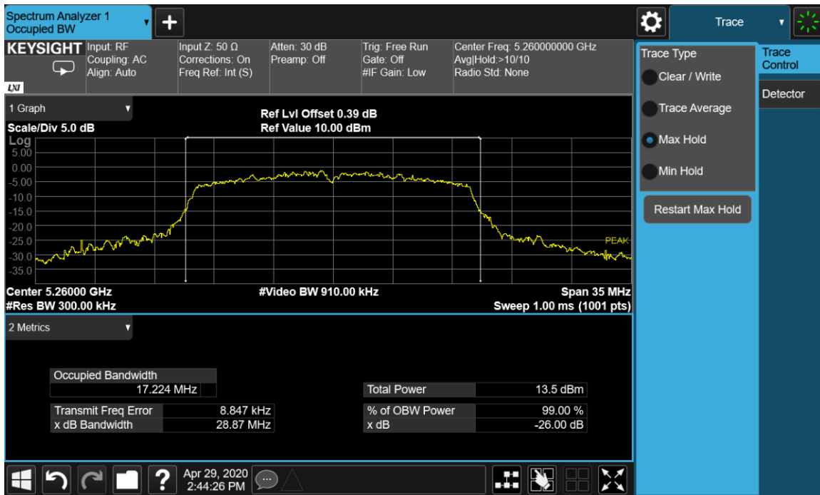
Plot 9-4. 26-dB Emission Bandwidth and 99% OBW Chain A 802.11a (Ch. 52)
