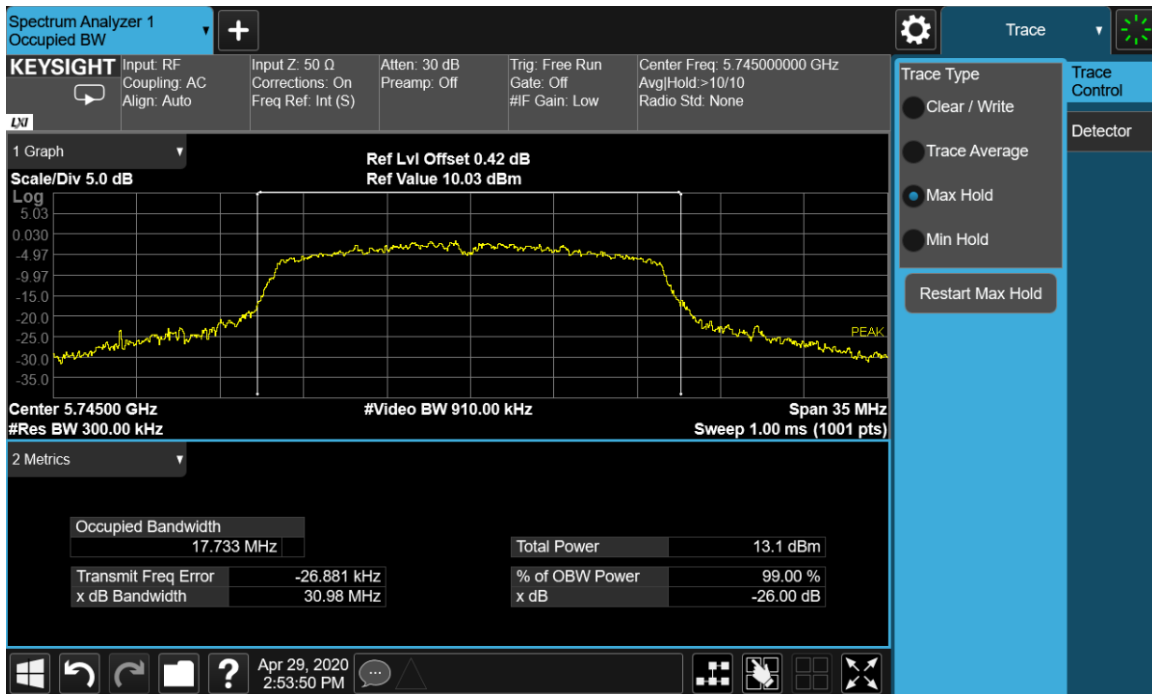
Plot 9-10. 26-dB Emission Bandwidth and 99% OBW Chain A 802.11a (Ch. 149)
