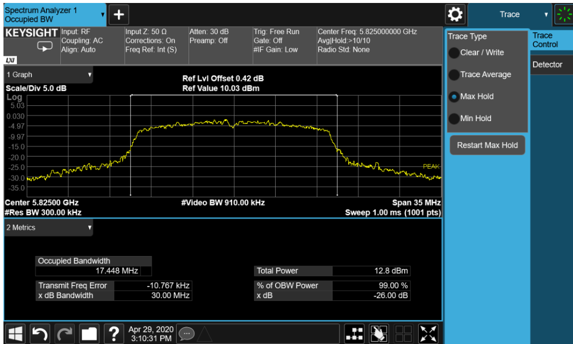
Plot 9-12. 26-dB Emission Bandwidth and 99% OBW Chain A 802.11a (Ch. 165)
