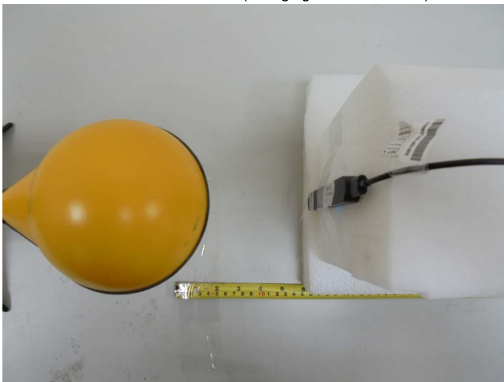
H-Field- Z-axis Bottom (Charging Mode with Load)
