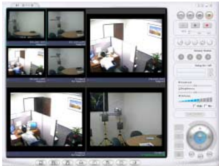
Figure 5-1. Select the display channel and click the “Camera Admin” button to log on to the administrative mode from “NVR100”
