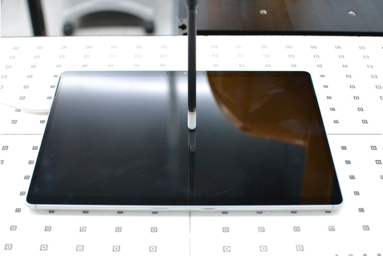
Figure E-3 Near Field Power Density Test Setup Photo – Front Side at 2mm
