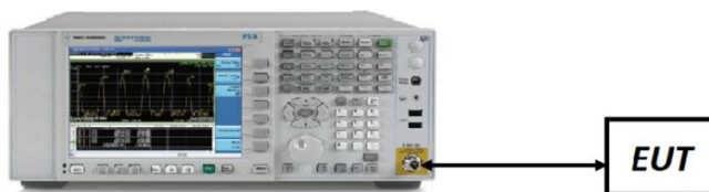
Figure 7-4. Test Instrument & Measurement Setup
