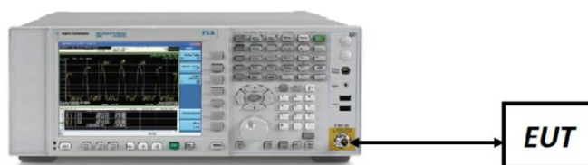
Figure 7-1. Test Instrument & Measurement Setup
