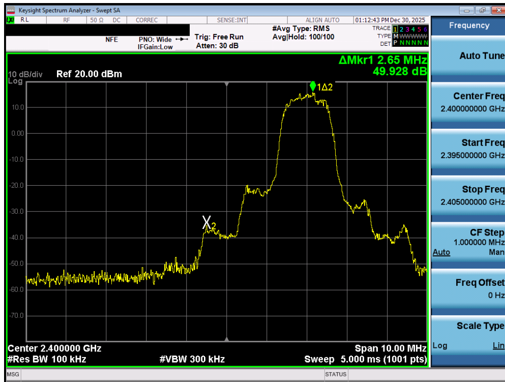
Plot 7-113. Band Edge Plot (Bluetooth with Hopping Disabled, 3 Mbps – Ch. 0) – SISO ANT2
