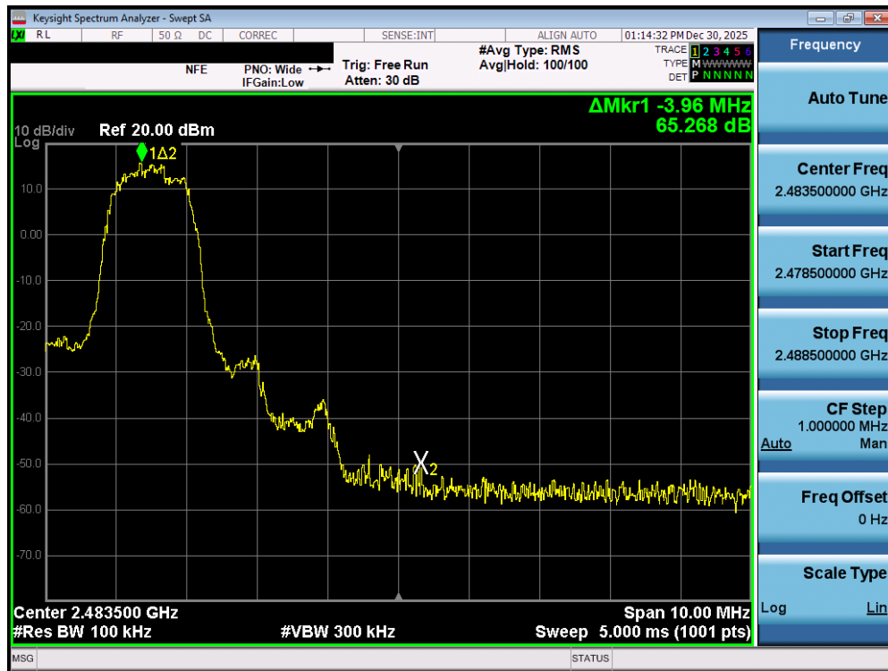
Plot 7-114. Band Edge Plot (Bluetooth with Hopping Disabled, 3 Mbps – Ch. 78) – SISO ANT2
