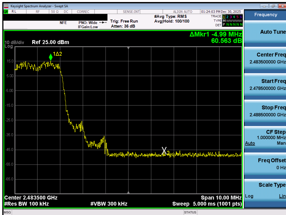
Plot 7-116. Band Edge Plot (Bluetooth with Hopping Enabled, 3 Mbps) – SISO ANT2
