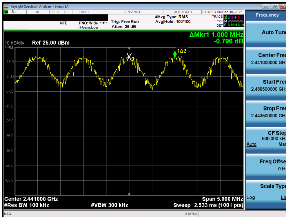
Plot 7-126. Channel Spacing Plot (Bluetooth) – SISO ANT2
