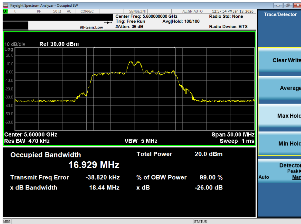
Plot 7-30. 26dB Bandwidth Plot MIMO ANT2 (20MHz BW 802.11be – 26 Tones (UNII Band 2C) – Ch. 120)
