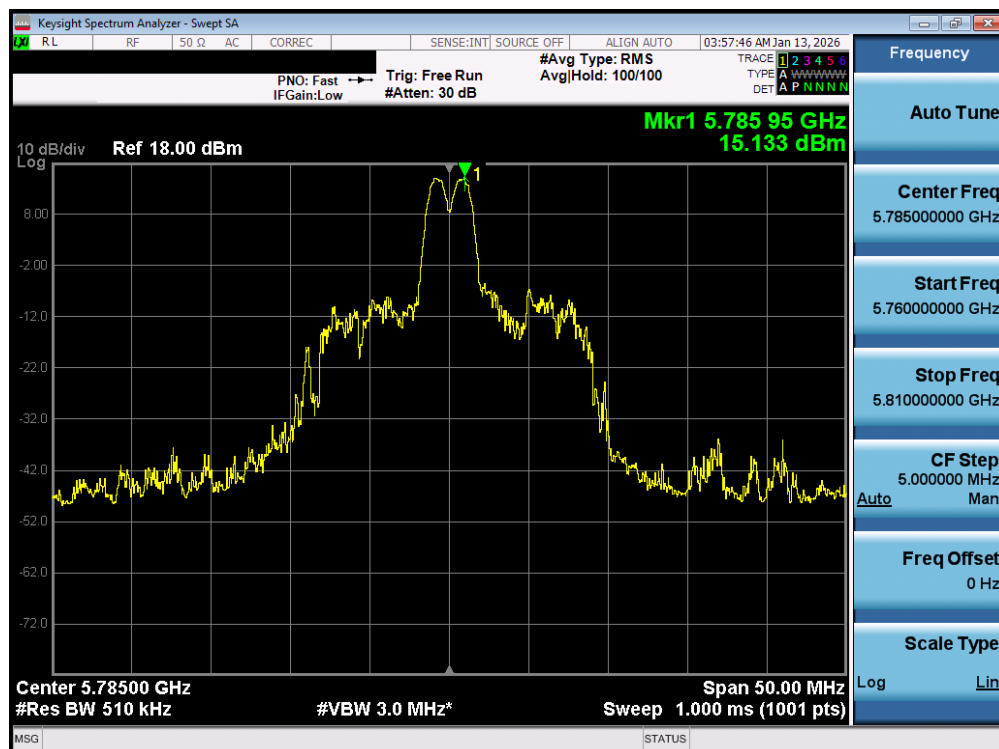
Plot 7-91. Power Spectral Density Plot MIMO ANT1 (20MHz BW 802.11be – 26 Tones (UNII Band 3) – Ch. 157)
