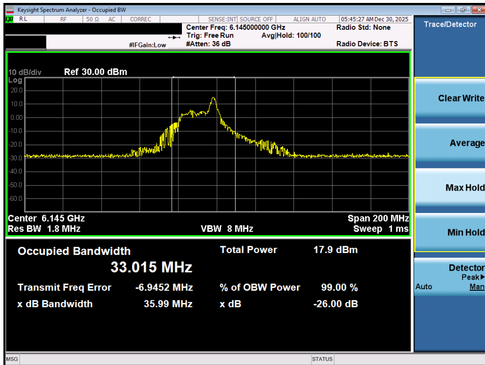
Plot 7-17. 26dB Bandwidth Plot MIMO ANT1 (80MHz 802.11ax/be (26 Tones) (UNII Band 5) – Ch. 39) - SP
