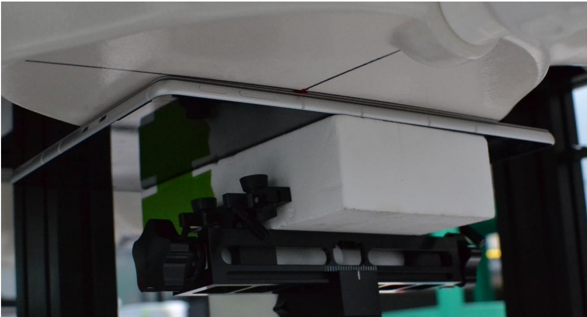
SAR Test Setup Photo 4 – Tablet, Back Side at 0mm – Antenna L
