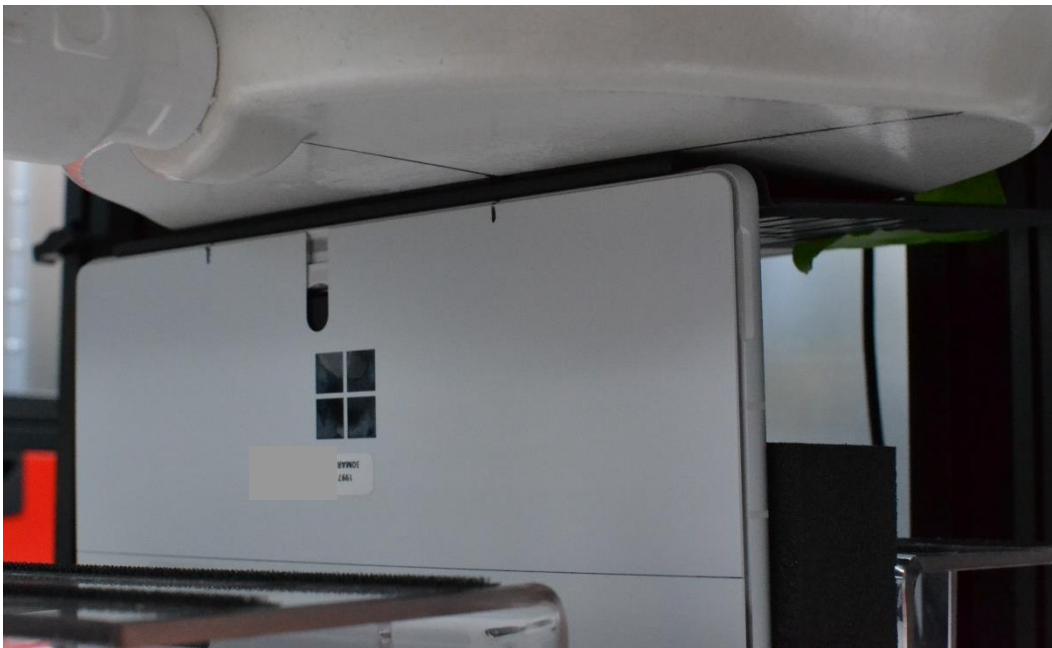
SAR Test Setup Photo 15 – Laptop, Bottom Edge at 0 mm – Antenna R
