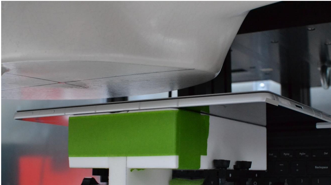
SAR Test Setup Photo 6 – Laptop, Back Side at 25mm – Antenna L
