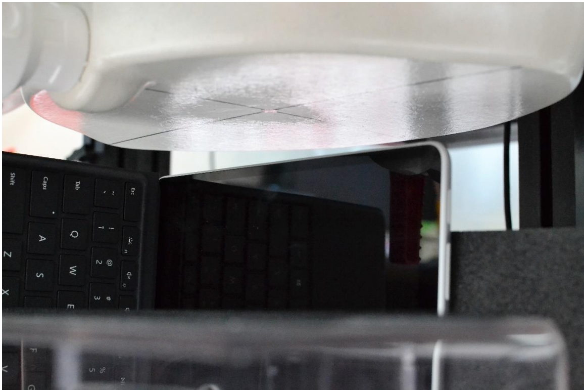
SAR Test Setup Photo 25 – Laptop, Left Edge at 25mm – Antenna R and Antenna L
