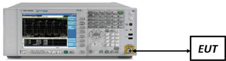
Figure 7-5. Conducted Test Setup > 1GHz
