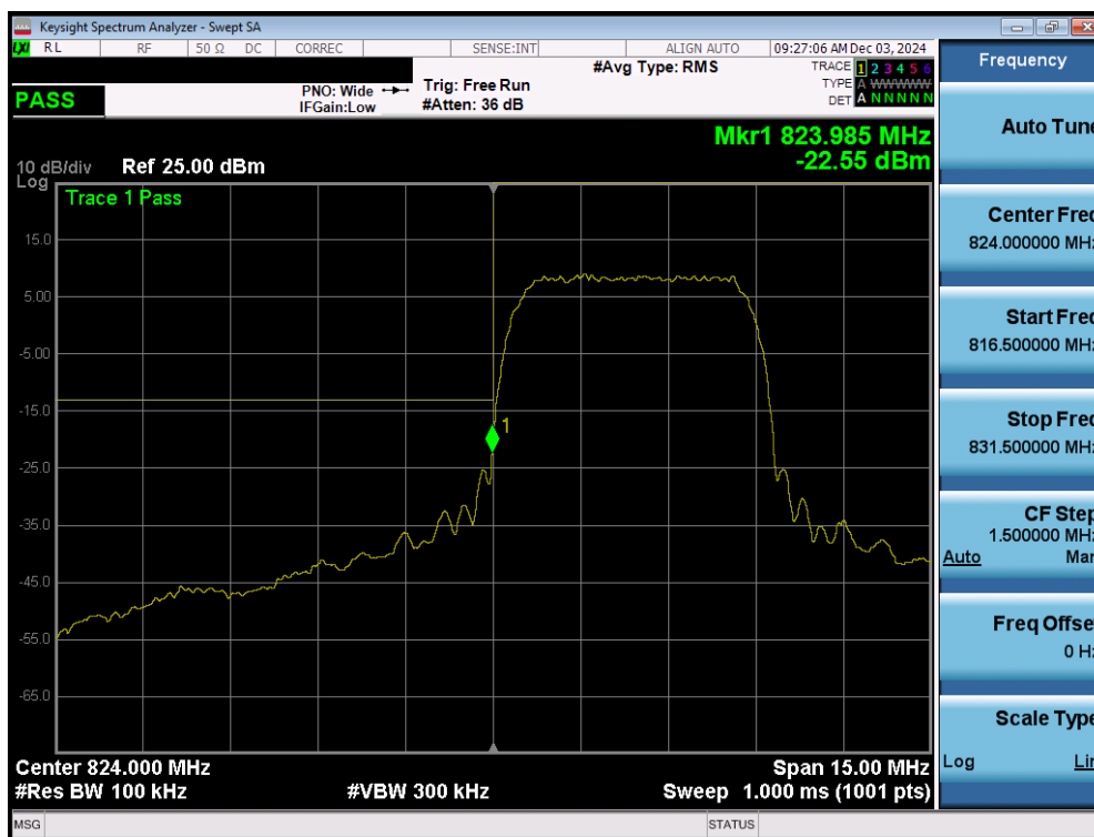
Plot 7-67. Lower Band Edge Plot (WCDMA Cell – Ch. 4132 – Ant 5)
