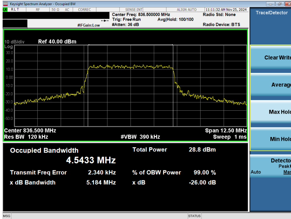
Plot 7-28. Occupied Bandwidth Plot (LTE Band 26/5 - 5MHz QPSK - Full RB - Ant 2)
