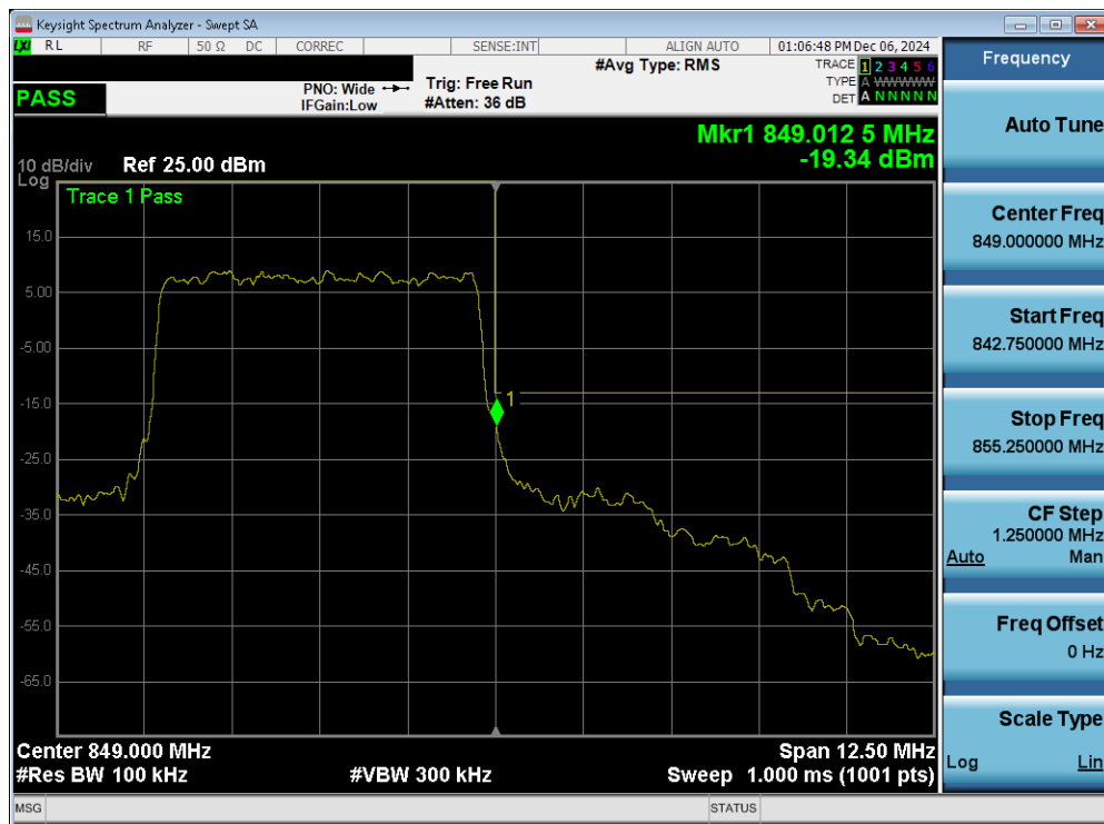
Plot 7-74. Upper Band Edge Plot (NR Band n5 – 5.0MHz - Full RB - Ant 5)
