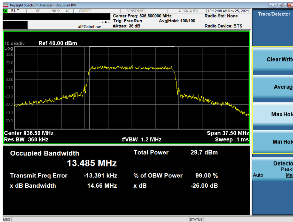
Plot 7-24. Occupied Bandwidth Plot (LTE Band 26 - 15MHz QPSK - Full RB - Ant 2)
