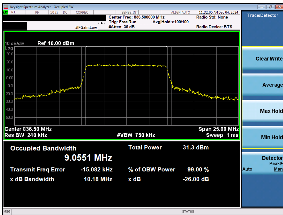
Plot 7-5. Occupied Bandwidth Plot (LTE Band 26/5 - 10MHz 16-QAM - Full RB - Ant 5)
