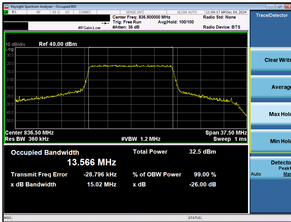
Plot 7-2. Occupied Bandwidth Plot (LTE Band 26 - 15MHz QPSK - Full RB - Ant 5)
