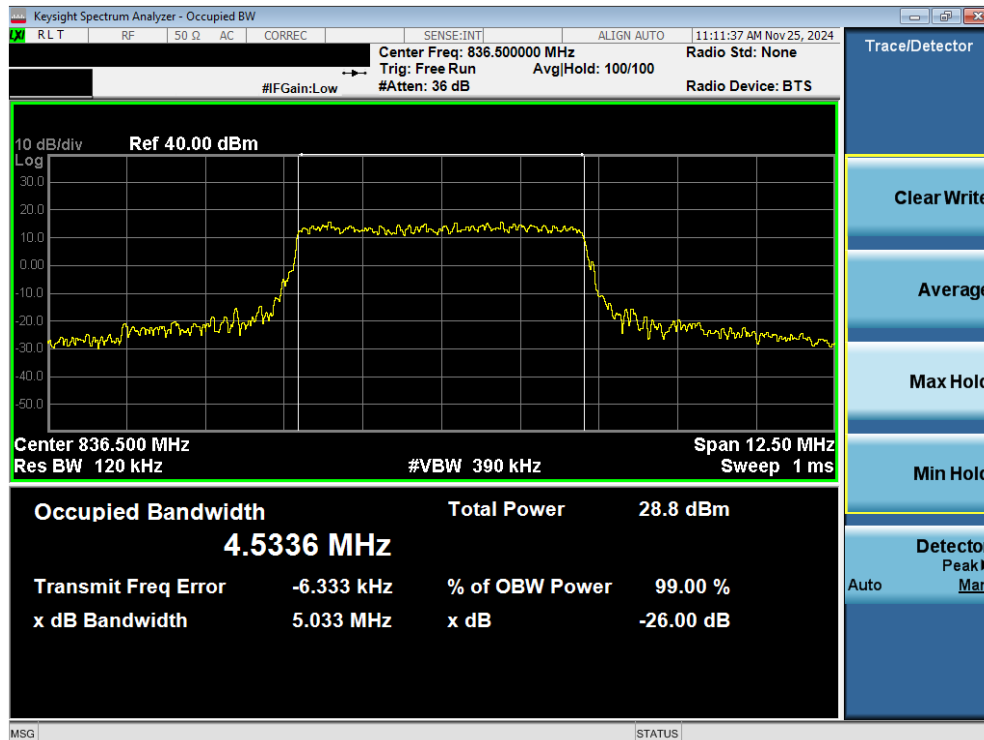
Plot 7-29. Occupied Bandwidth Plot (LTE Band 26/5 - 5MHz 16-QAM - Full RB - Ant 2)
