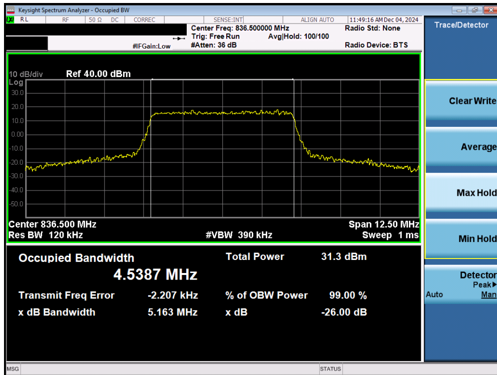
Plot 7-7. Occupied Bandwidth Plot (LTE Band 26/5 - 5MHz 16-QAM - Full RB - Ant 5)
