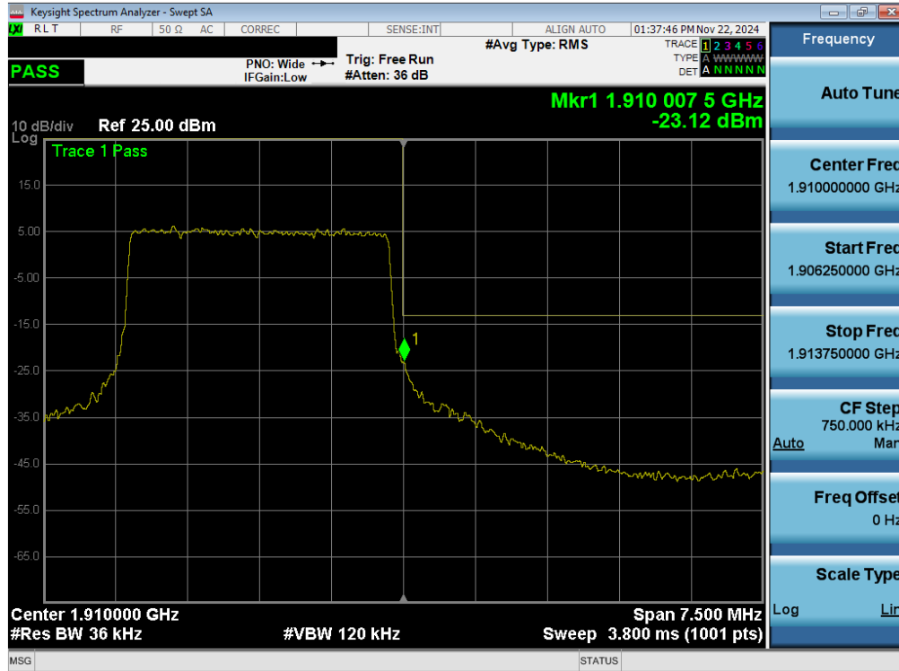
Plot 7-56. Upper Band Edge Plot (LTE Band 2 - 3MHz QPSK – Full RB - Ant 1)
