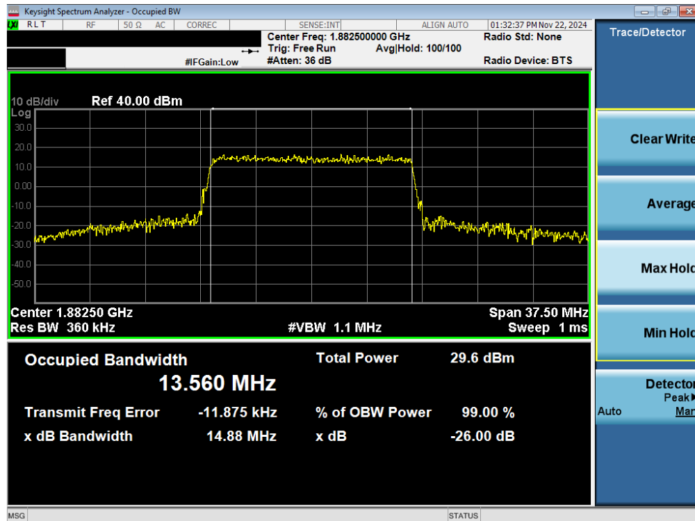
Plot 7-5. Occupied Bandwidth Plot (LTE Band 25/2 - 15MHz 16-QAM - Full RB - Ant 1)
