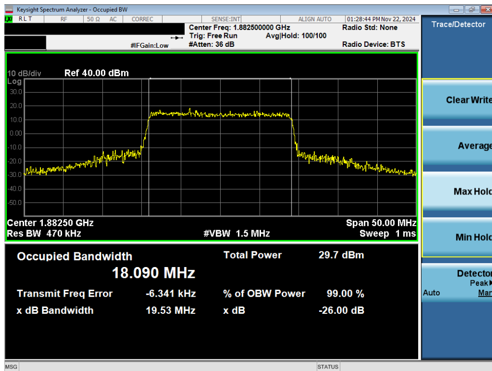
Plot 7-3. Occupied Bandwidth Plot (LTE Band 25/2 - 20MHz 16-QAM - Full RB - Ant 1)
