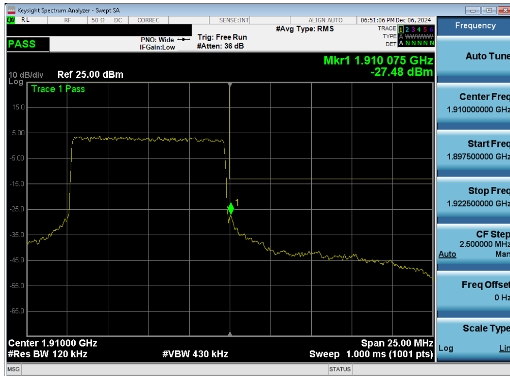
Plot 7-66. Upper Band Edge Plot (NR Band n2 - 10MHz QPSK – Full RB - Ant 1)
