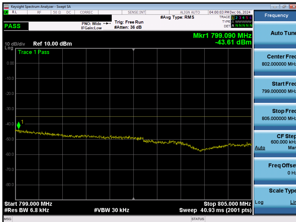
Plot 7-124. Upper Emission Mask Plot (LTE Band 14, 5MHz QPSK - RB Size 25 – Ant2)
