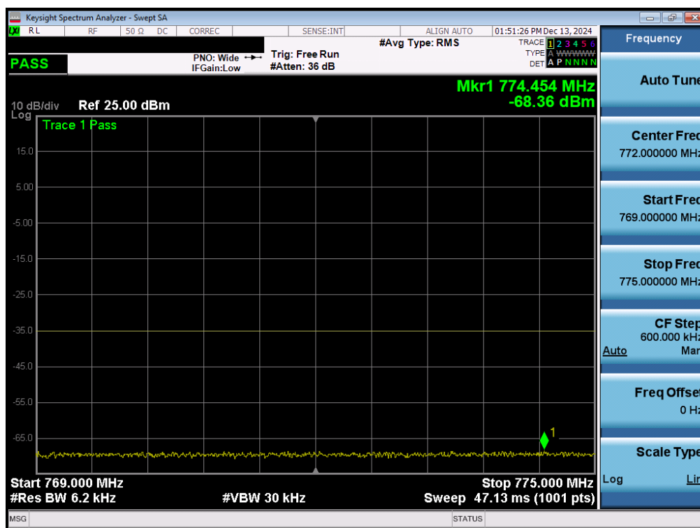
Plot 7-116. Lower Emission Mask Plot (NR Band n14, 5MHz QPSK - RB Size 25 – Ant5)
