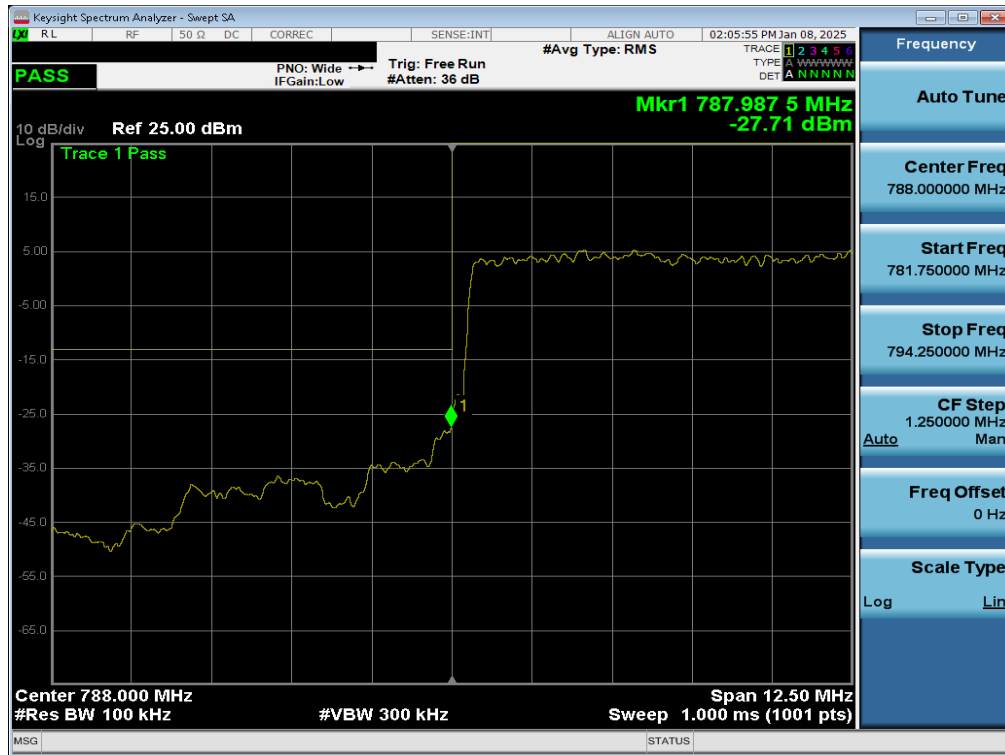
Plot 7-127. Lower Band Edge Plot (NR Band n14, 10MHz QPSK - RB Size 50 – Ant2)
