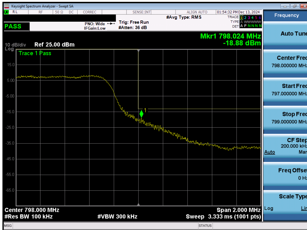
Plot 7-117. Upper Band Edge Plot (NR Band n14, 5MHz QPSK - RB Size 25 – Ant5)
