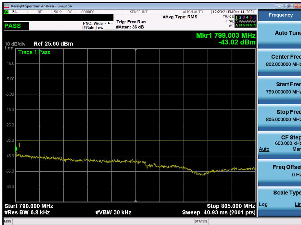
Plot 7-112. Upper Emission Mask Plot (LTE Band 14, 5MHz QPSK - RB Size 25 – Ant5)
