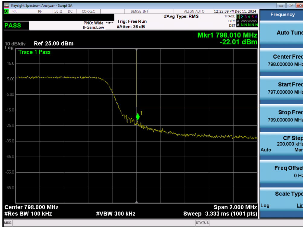
Plot 7-111. Upper Band Edge Plot (LTE Band 14, 5MHz QPSK - RB Size 25 – Ant5)
