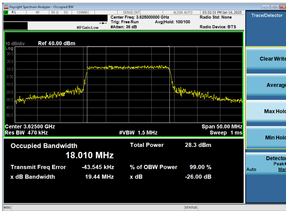
Plot 7-33. Occupied Bandwidth Plot (LTE Band 48 - 20MHz 16-QAM - Full RB Configuration - Ant1)
