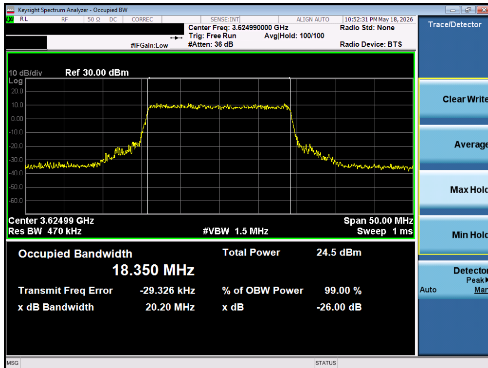
Plot 7-47. Occupied Bandwidth Plot (NR Band n48 - 20MHz QPSK - Full RB Configuration - Ant6)
