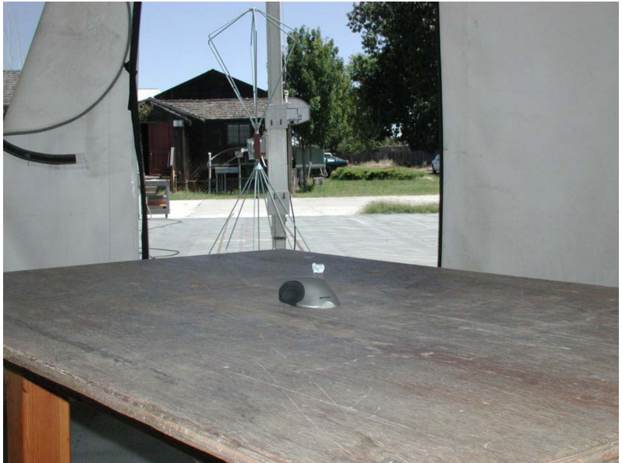
Photo 3 – Test Setup at Compliance Certification Services OATS (30MHz 1GHz)
