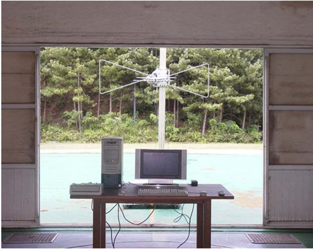
Radiated Emissions - Front View
