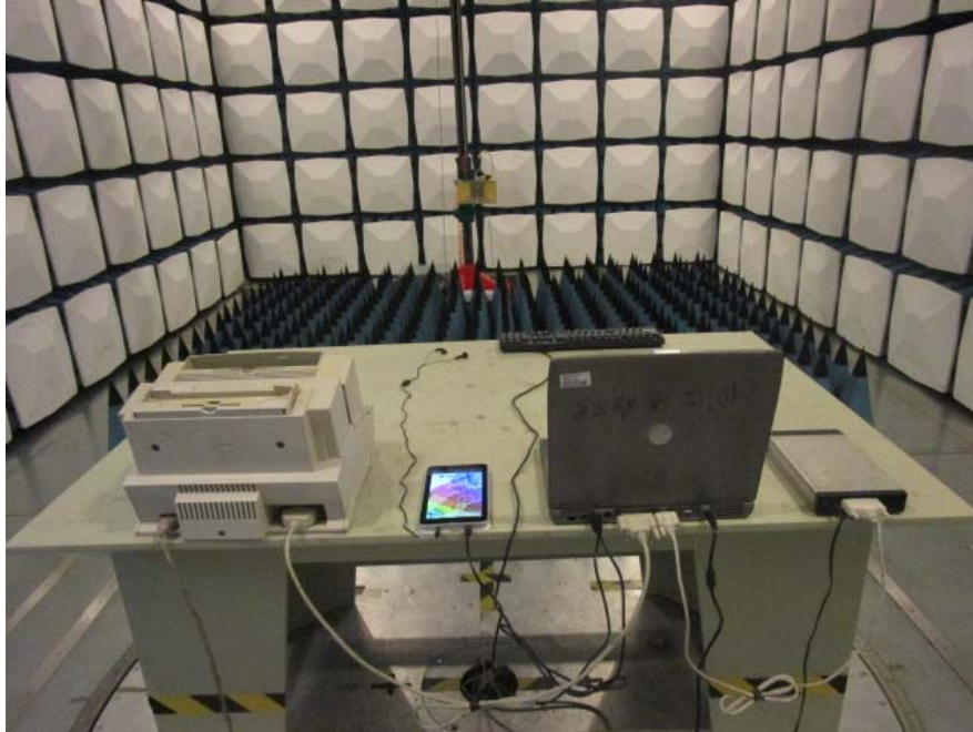
Radiated Emission –Rear View (Above 1 GHz)
