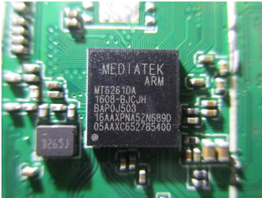
EUT –Main Chip View
